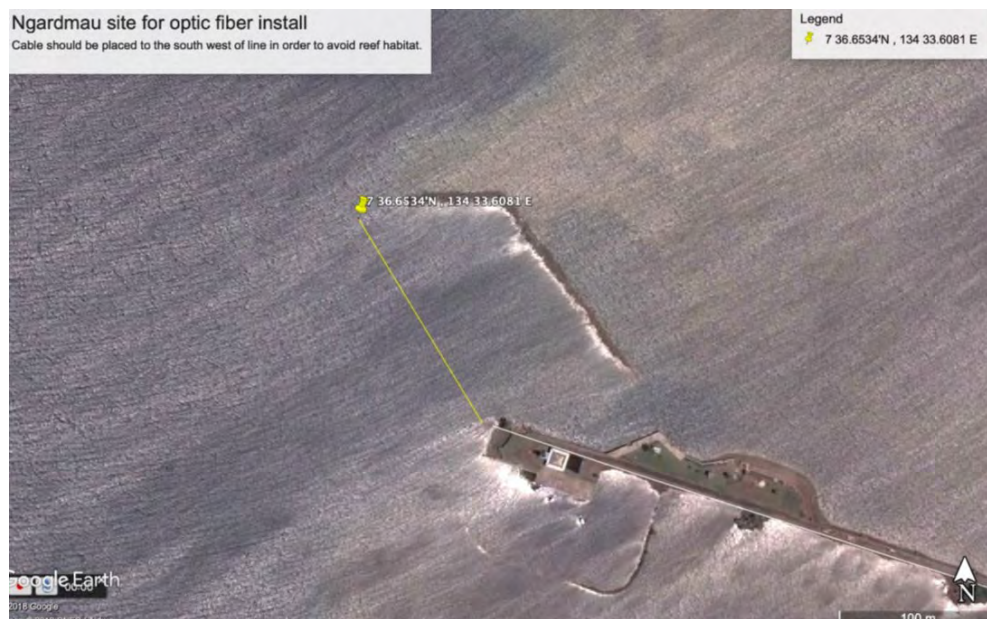
Figure 1: Cable route alignment
